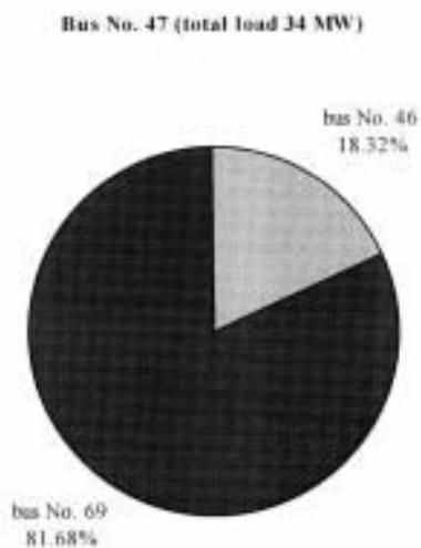
Fig. 5. Generators' contributions to the bus no. 47 active power demand after a customer at the bus no. 54 purchase additional 100 MW from the power plant at the bus no. 46.
